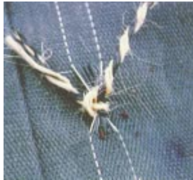
▲ Geolon fabric with loops to which weips are secured.
