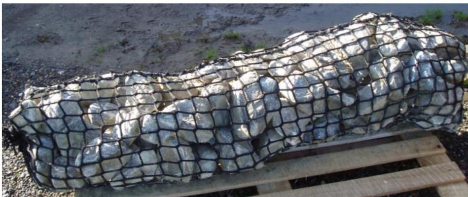
Rock Rolls that are installed below coir units can also be used to support a filter fabric or biodegradable matting. This system retains the fines in the bank while the roots of the plants from the pre-vegetated coir units establish themselves into the bed of the waterway and through the woven geotextile into the suitable fill.
